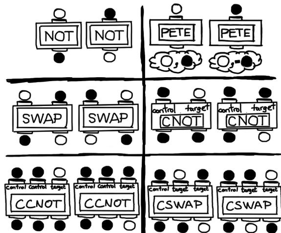
In the diagram, only cases where the output is different from the input are shown—in all other cases the boxes do not change the input.
